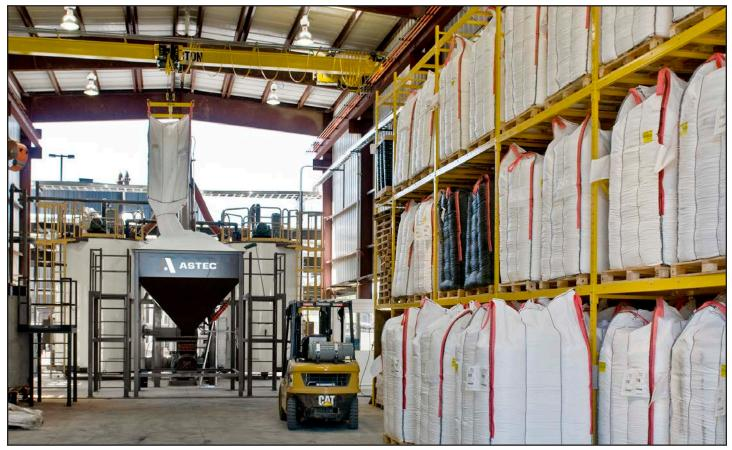
At this terminal polymer pellets are purchased in Super Bags and are stored on shelves shown here. The bags are easily accessed by a trolley that transports them to the hopper for unloading. This system eliminates the need for a lift truck and box dumper.
