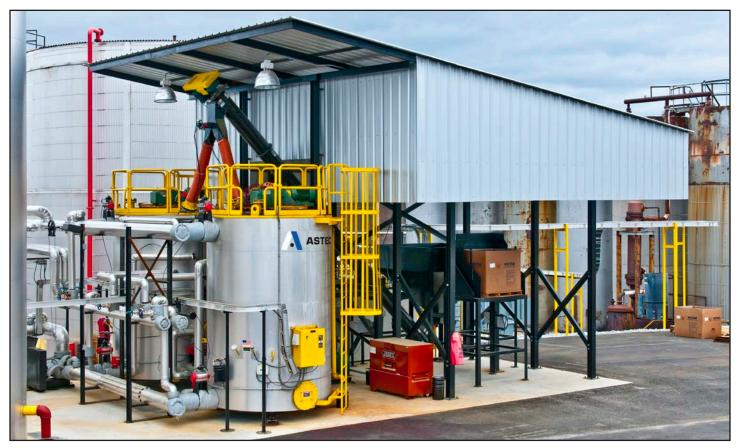
Two mixing tanks are shown on the left side of the photo. A hopper and box dumper is shown under the covered area.
