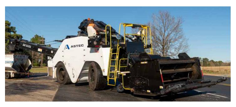
The dump truck is not able to maneuver into the intersection of this jobsite. The SB-3000 solves this problem. The mix is dumped from the dump truck into the SB-3000's hopper and shuttled to the intersection where it is placed into the waiting paver.
