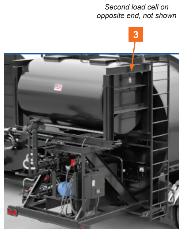
Horizontal Calibration Tank installed on a Heli-Tank
