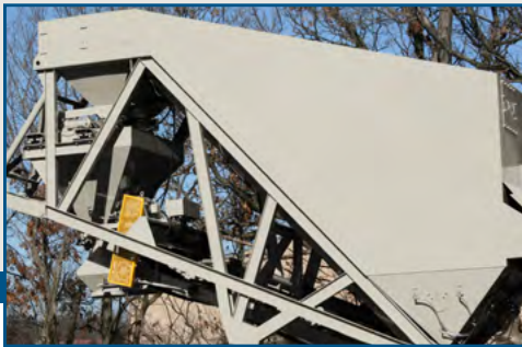
225 BBL Silo with Gravity Feed Surge Hopper
