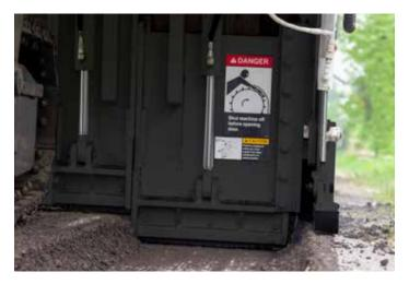
Variable Cutter System: VCS<sup>®</sup> allows the change of cut widths by only changing the drum.
