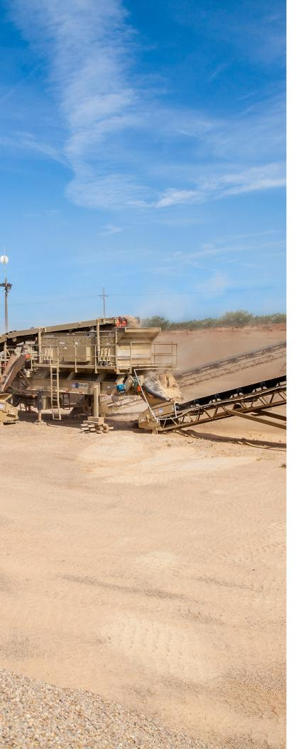
Harvey uses the GT205S to process concrete rock and hot-mix material. By utilizing three screen decks, he is able to make A4 rock, a size of material the company previously had to discard. Now, Big Creek Sand and Gravel is able to avoid wasting material and can offer more products to its customers, he said.
