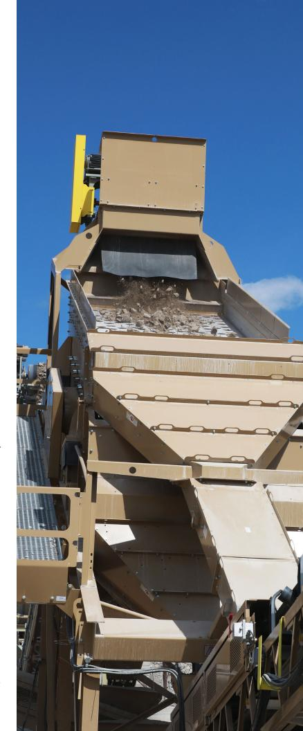
crushing performance and efficiency. Operators can initiate an automated calibration process via the touch screen monitor, that automatically "zero's-out" and resets to the proper setting. Operators can also modify the crusher setting at any time, even while crushing.
