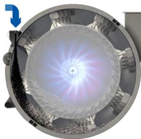
Liquid asphalt is injected into the mixing chamber through the AC inlet or optional warm mix system
