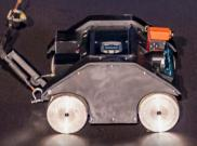
Test silo wall thickness without sending anyone into the silo. Astec SiloBot inspection service uses an innovative wireless remotely controlled robot that analyzes, evaluates and inspects asphalt silos for imperfections.
