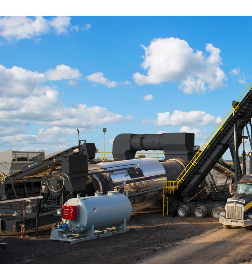
The standard setup comes with the drum mixer, cold feed, scalping screen (with inclined conveyor), baghouse, surge bin, drag conveyor and control house. The baghouse load also holds the inertial dust collector. One load handles the SEB and drag conveyor. All ship with ductwork, dust screws, electrical switch gear, cables, and plant controls. Astec also supplies RAP bins, fuel tanks, lime mixers and AC tanks.
